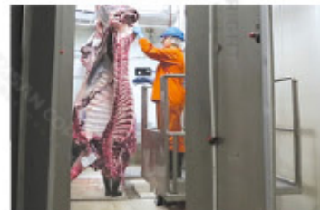
VETERINARY CONTROL The carcass, liver, head and tripe of the same animal meet at the same point and controlled by the veterinary. The animal diagnosed to be suspicious is strayed from the line and directed to the suspicious cold room.
