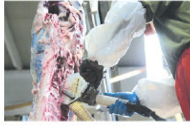
SPINAL CORD VACUUMING In this unit, the spinal cord and nerves of the animal are removed with a spinal cord vacuum machine. In this way, bacteria formation is prevented and the usage life of the quality meat is extended.
