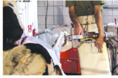
FOOT and HORN CUTTING The feet and horns are cut using a pair of hydraulic scissors at the end of the bleeding line and before the processing, the processing line starts at the stage platform with a transfer between the rails.
