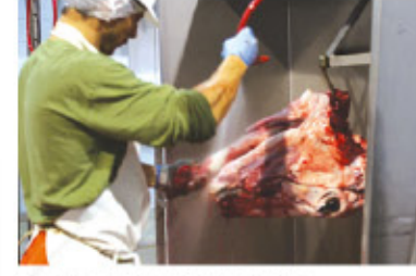
HEAD CLEANING CABIN In this cabin skinned head is cleaned before transfer to veterinary control point and to the offal room.
