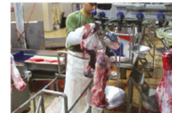
LIVER EXTRACTING The liver and internal organs of the animal are extracted and hanged to the liver conveyor. The parts are transferred to the internal organ room without manual interference.
