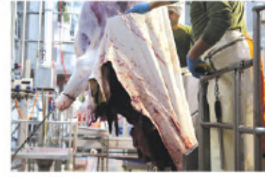
DEHIDING In this section, integrated dehiding machine, movable drum and movable platforms on both sides are used together. The butchers on the platform take their positions and prevent the meat from breaking during the dehiding operation.
