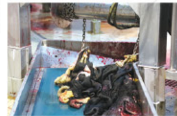
SKIN TRANSFERRING CONVEYOR Transfers the skin to the skin section through a conveyor line without manual interference and without damaging the skin.
