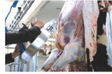
BRISKET OPENING In this unit, a brisket opening saw is used and the chest part of the carcass is opened to ensure the internal organs removed easily along the line.
