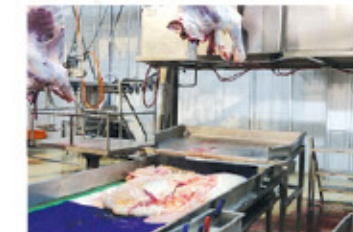
TRIPLE TRANSFERRING CONVEYOR The tripe is transferred to the offal room without manual interference with the help of an automatic band conveyor.
