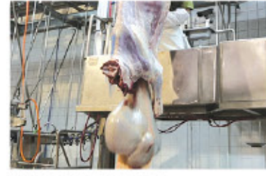
TRIPLE EXTRACTING The tripe and intestine are extracted from the chest and dropped on the automatic tripe band conveyor; passes through the veterinary control point and carried automatically without human interference to the offal room.
